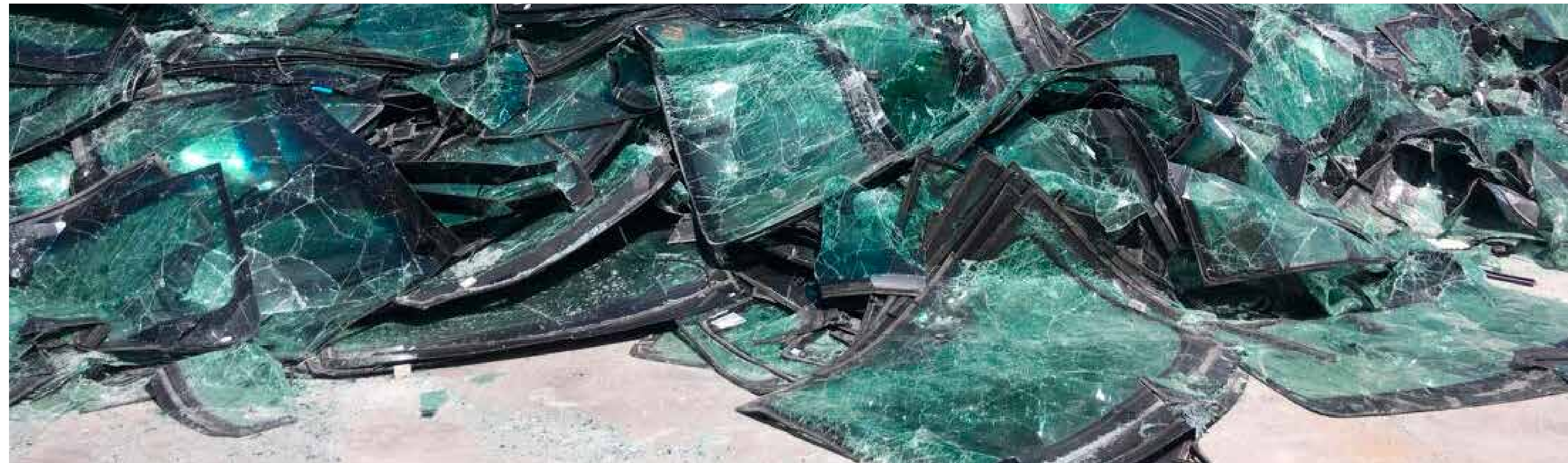
From broken windshields to sustainable carpet backings: we introduced PVB dispersion as a binder in carpet pre-coat and backings. It is an important solution for utilizing post-consumer materials such as recycled windshields and architectural glass) in the carpet industry.
